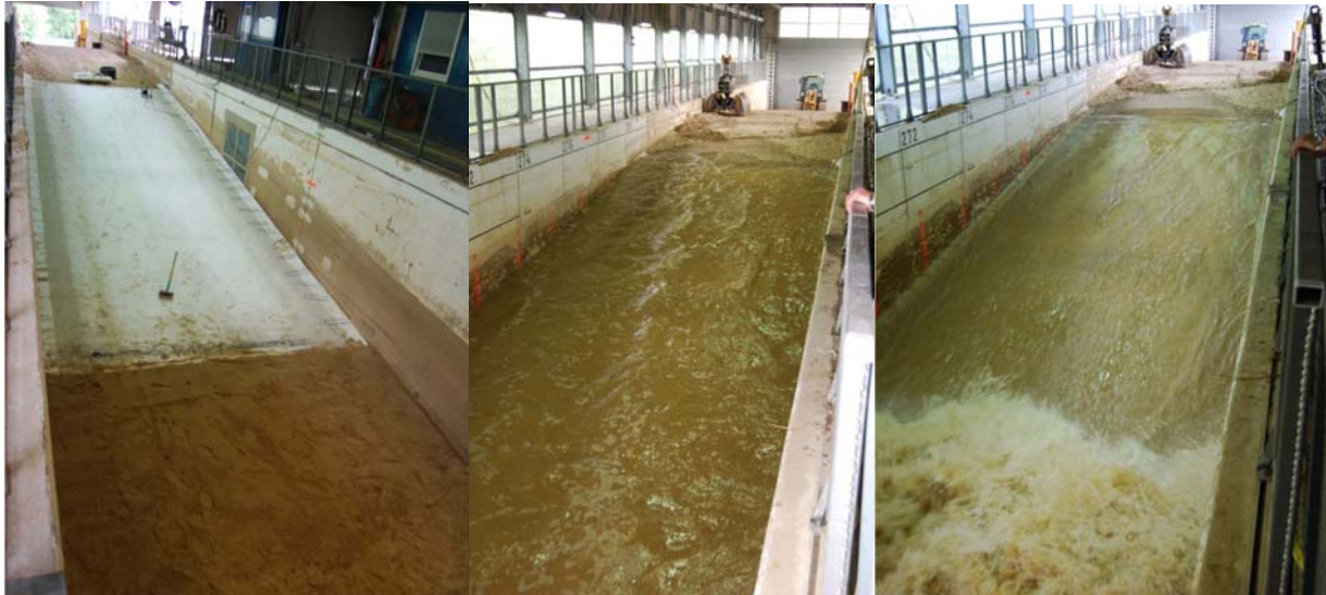
Figure 10: Physical model tests under wave loads – Hydraulic stability of the heavy composite GCL under wave loads (FZK, 2009)
