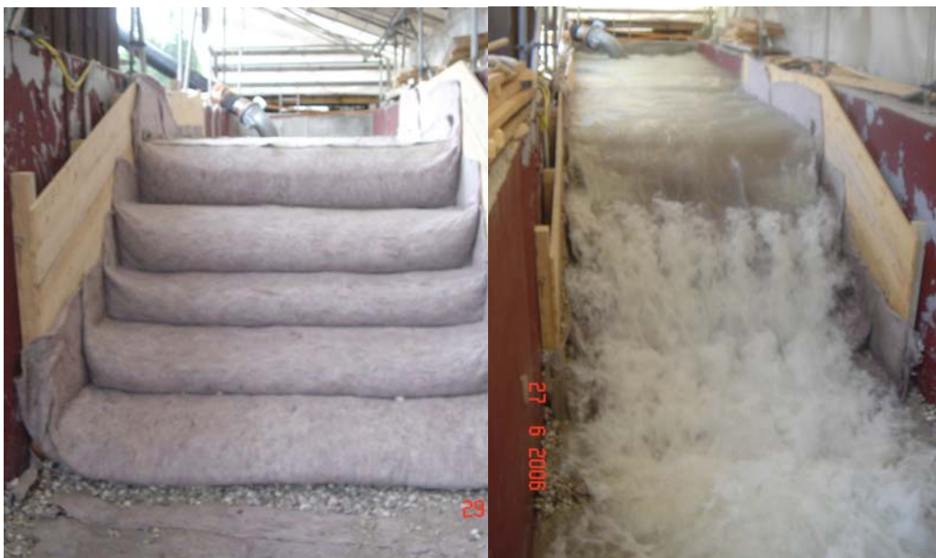
Fig. 11 Model experiments at the Technical University Munich, Overflow of the inner embankment per method (III). Left: before overflow, right: in overflow state with up to 130 l/m-s (Haselsteiner et al. 2007)
