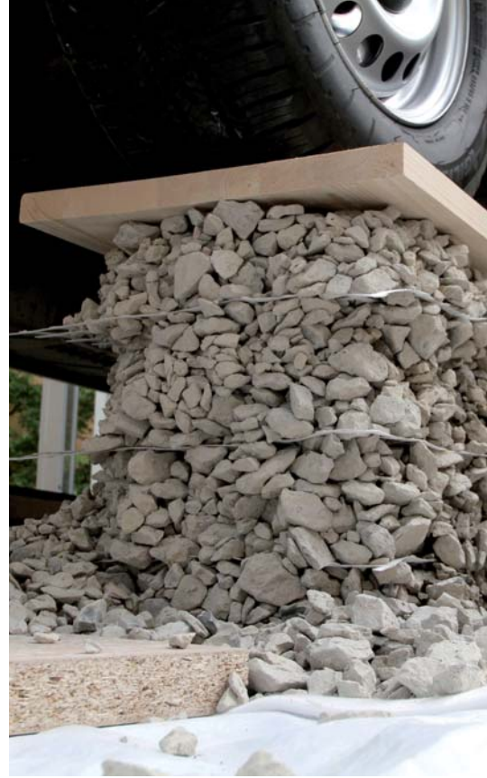
Figure 2 Lateral restraint of base course aggregate with Secugrid® geogrids
