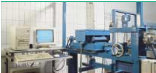
Direct shear device for the determination of friction coefficients (EN ISO 12957 T1)
