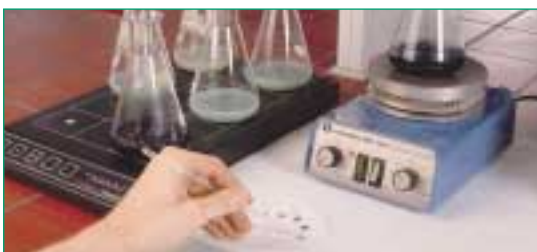
Determination of the montmorillonite content of bentonite via the methylene-blue-adsorption (titration) method
