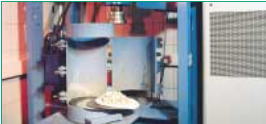
Load plate-bearing test for the qualification of geotextile protection layers (EN 13719)
