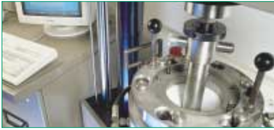
Static puncture test according to EN ISO 12236
