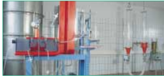
Determination of the hydraulic properties of water permeable geosynthetics
