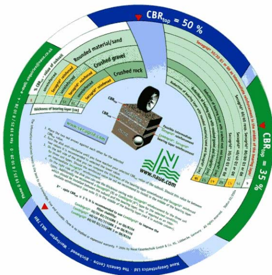
Fig. 3: Design disc for bearing layer reinforcement in traffic areas using welded Secugrid® geogrids
