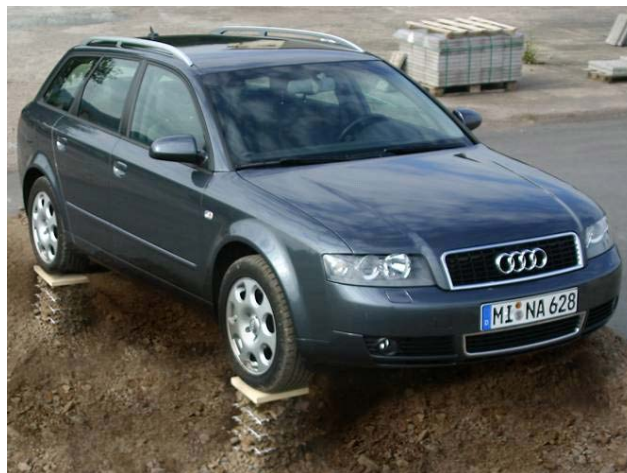
Fig. 1: Geogrid reinforced gravel columns carrying a car
