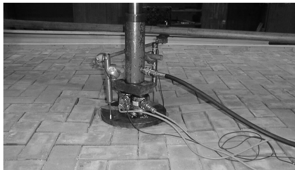
Figure 9.13.7 Testing of a full-scale pavement incorporating a plastic cellular sub-base replacement system
