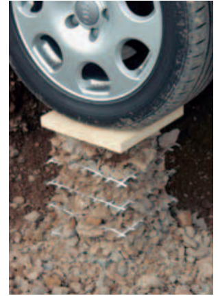
Fig. 2 Demonstration of the interlock effect with a car standing on a Secugrid® reinforced gravel column
